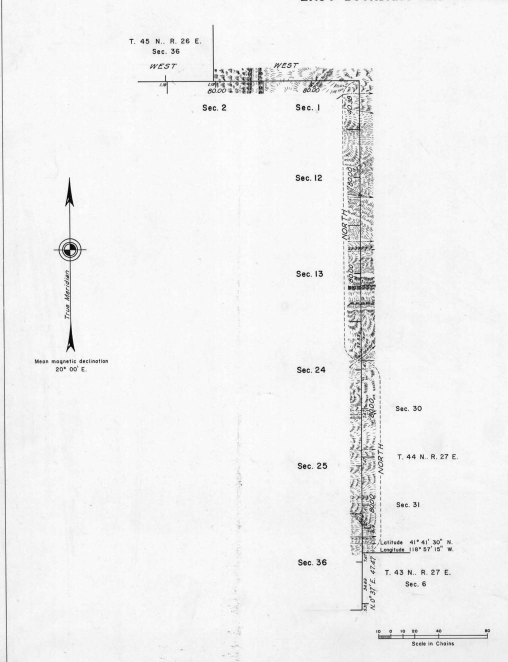
This plat represents the dependent resurvey of a portion of the west boundaries of Ts. 43 and 44 N., R. 27 E., designed to restore all corners in their true original locations according to the best available evidence, and the survey of the east boundary and a portion of the north boundary of T. 44 N., R. 26 E., M.D.M., Nevada.
