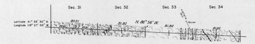
This plat represents a dependent resurvey of a portion of the south boundary designed to restore all corners in their true original location according to the best available evidence.
