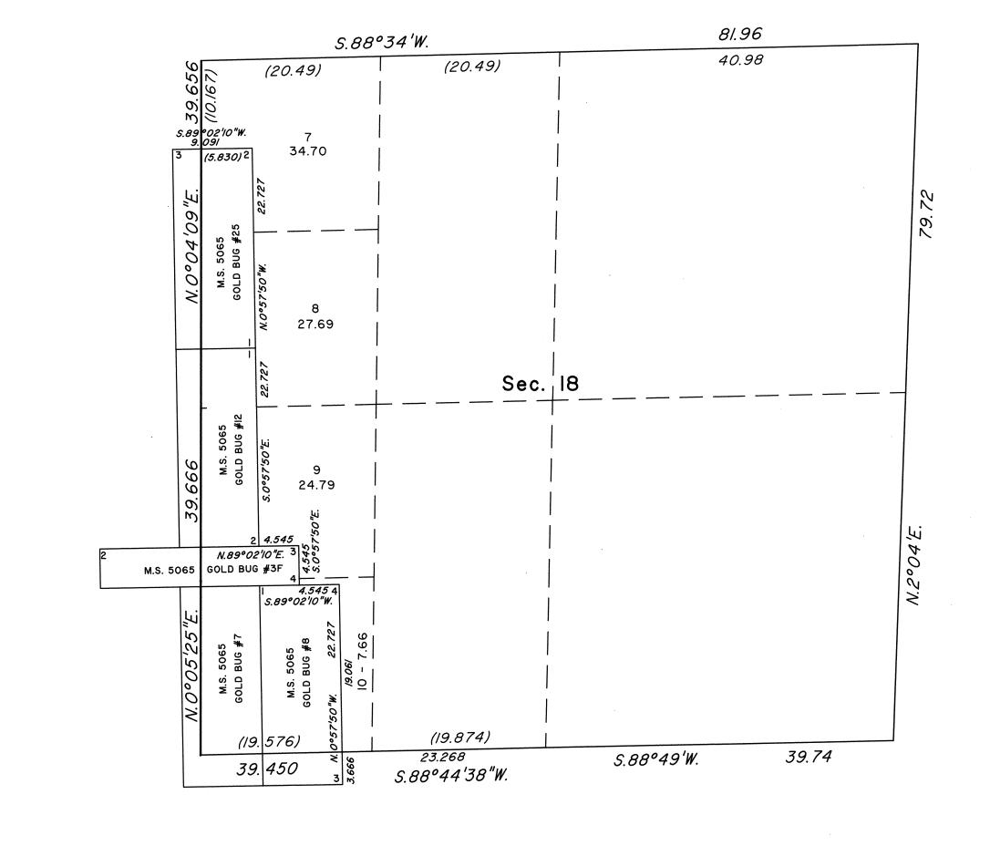
This plat, showing amended lottings created by the segregation of Mineral Survey No. 5065 in section 18, T. 36 N., R. 50 E., Mount Diablo Meridian, Nevada, is based on the plats approved February 13, 1873 and January 13, 1885, the plat accepted April 3, 1987, and the mineral survey records.
