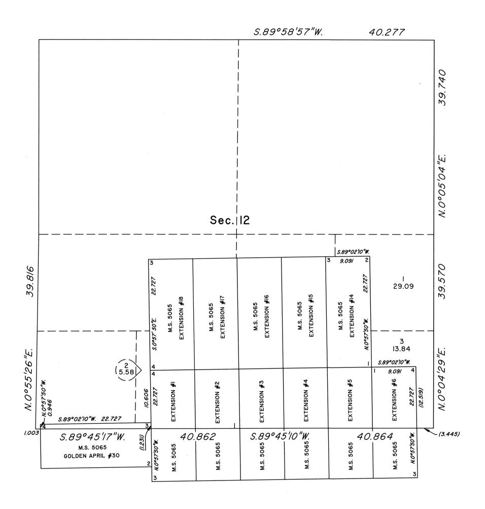
This plat, showing new lottings created by the segregation of Mineral Survey No. 5065 in section I2, T.36N., R.49E., Mount Diablo Meridian, Nevada, is based on the plat approved February I3, 1873, and the mineral survey records.
