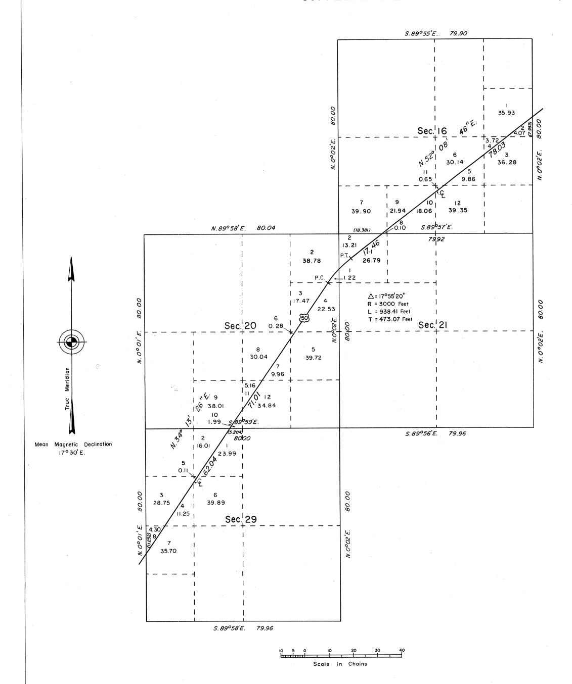
This supplemental plat of sections 16, 20, 21, and 29, T. 33 N., R. 70 E., Mount Diablo Meridian, Nevada, showing a subdivision of certain quarter quarter sections into separate areas bounded by the centerline of the highway, is based upon the plat accepted August 13, 1948, and supplemental data on the highway centerline obtained from Nevada State Highway Department right-of-way applications, Nevada 041037, dated July 15, 1955, and amended May 31, 1966.
