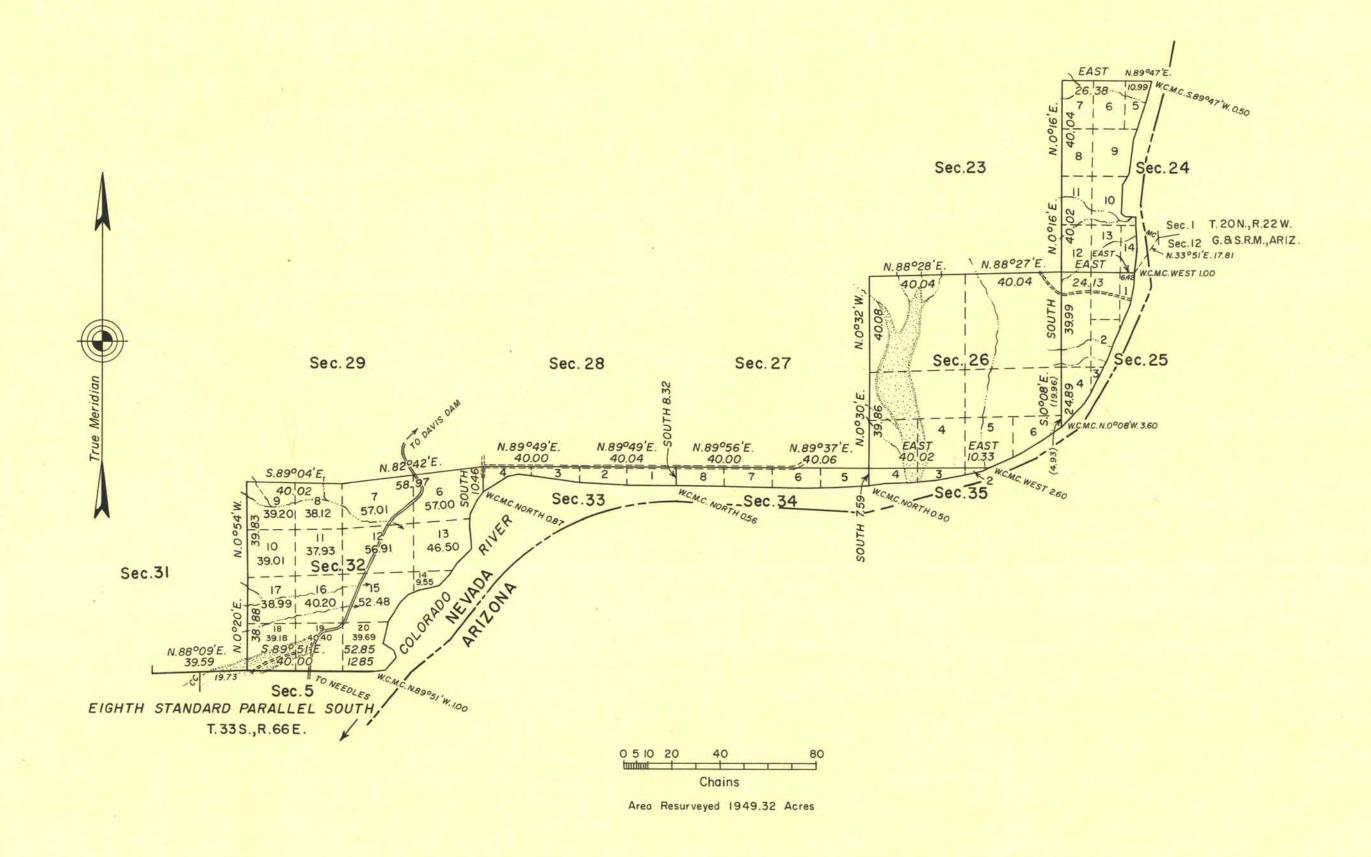
This plat represents a retracement and reestablishment of a portion of the Eighth Standard Parallel South and of a portion of the subdivisional lines designed to restore the corners thereof in their original positions according to the best available evidence.
