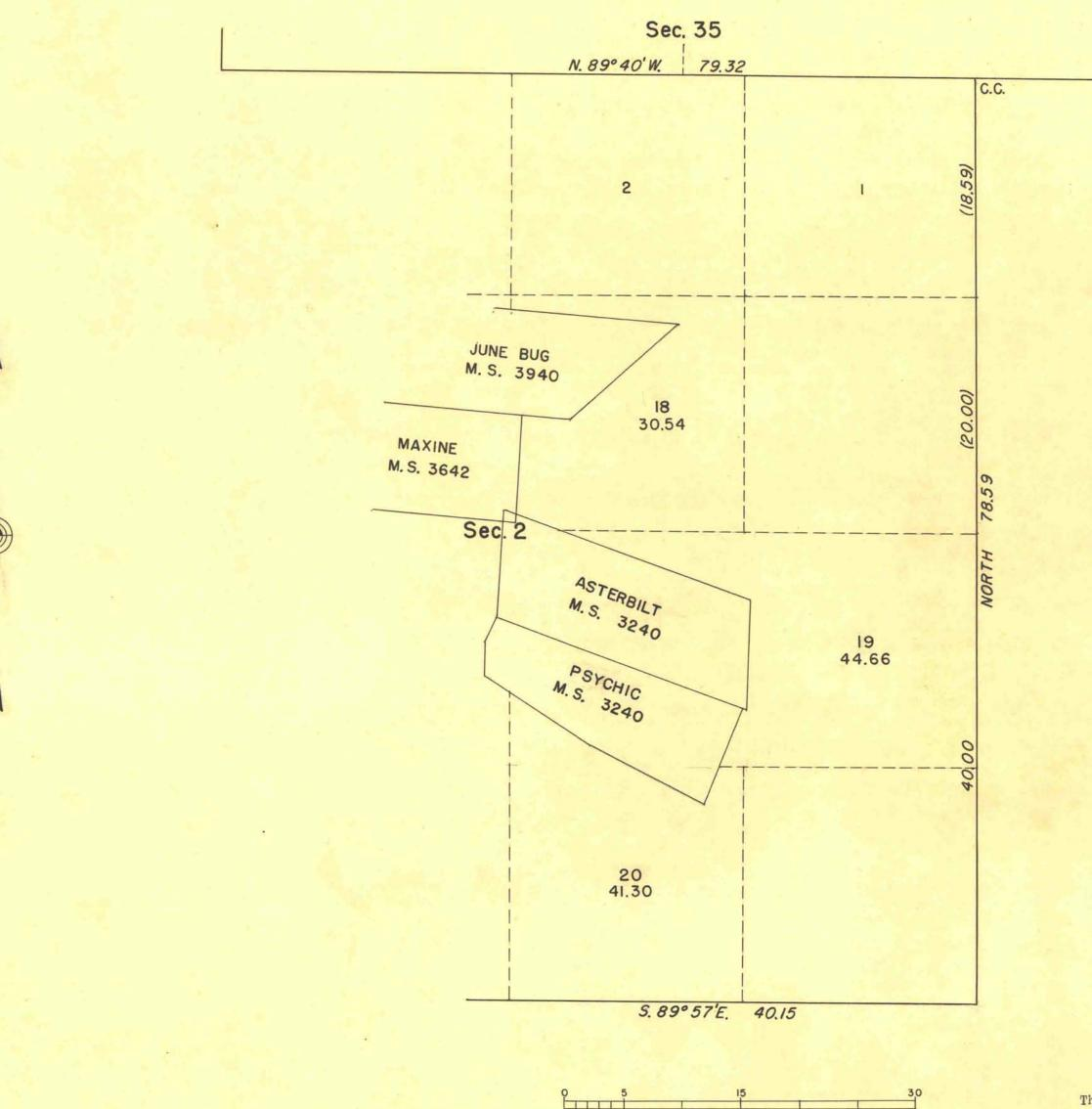
This supplemental plat showing revised lottings of the public land remaining in the east half of sec. 2 is based upon the plat of survey of T. 29 S., R. 63 E., approved February 23, 1884, the plat of the dependent resurvey of T. 28 S., R. 63 E., approved March 7, 1947 and accepted September 17, 1947, and upon the official mineral survey records.
