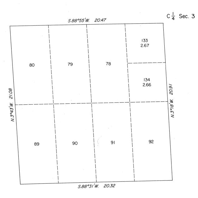
0 | 2 3 4 5 | 10 | Scale in Chains This plat showing a subdivision of original lot 77, sec. 3, T. 21 S., R. 60 E., Mount Diablo Meridian, Nevada, is based upon the plat accepted June 8, 1953.
