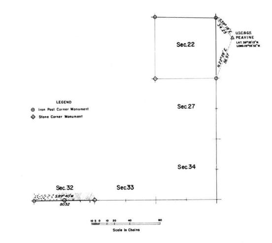
This plat represents the dependent resurvey of the south boundary of section 32 designed to restore the corners in their original locations according to the best available evidence, and the remonumentation of the section corners of section 22.
