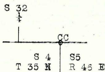
dig pits, 24x18x12 ins., crosswise on each line, E. and W., 3 ft., and S. of post, 7 ft. dist.; and raise a mound of earth, 4 ft. base, 2 ft. high, S. of cor.
