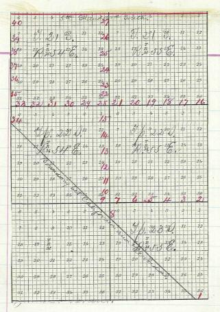
Survey made with Burt's Patent Improved Solar Compass, nearly new, and in first rate order. Made by M. G. L. Gurley of Gray N. J. in 1881 Before proceeding further with the exteriors of this Tp., I carefully examined the adjustments of my solar compass to day, particularly the latitude and reversing apparatus, and found them correct.
